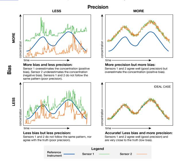
Figure 3-4. Illustration of Air Sensor Bias, Accuracy, and Precision
