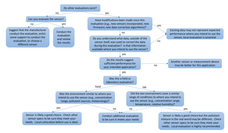
Figure 4-3. Flow Chart for Considering an Air Sensor Based on Performance
