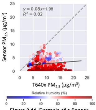
Figure 3-11. Example of a Sensor That Shows No Agreement with the Reference Instrument
