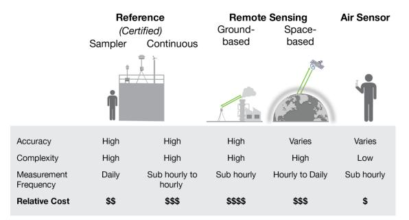
Figure 2-8. Common Types of Air Monitoring Instruments and Their Characteristics
