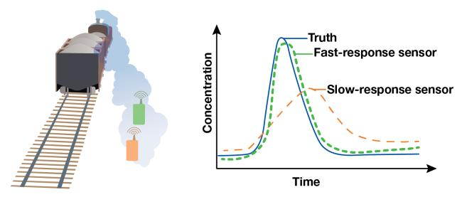
Figure 3-6. Example of an Air Sensor's Response Time
