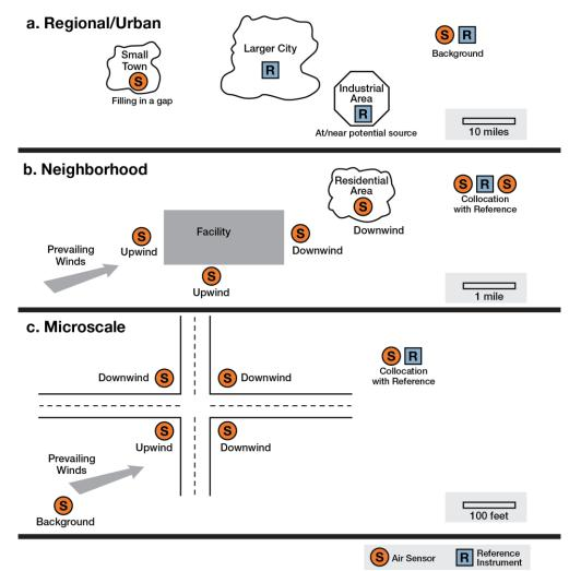
Figure 3-8. Example Maps for Placing Air Sensors for Networks of Different Scales Depending on the Purpose: a) Regional/Urban Network, b) Neighborhood Network, and c) Microscale, Small Area Network
