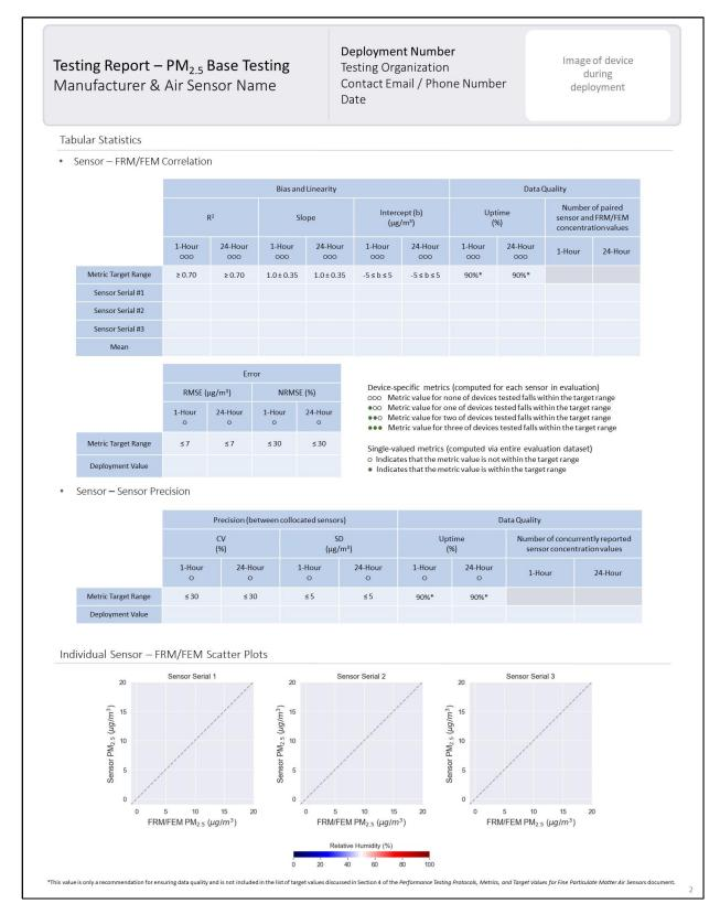
Figure E-2. Page 2 of U.S. EPA's Base Testing Reporting Template for PM<sub>2.5</sub> Sensors – Tables and Graphs Summarizing Sensor Performance
