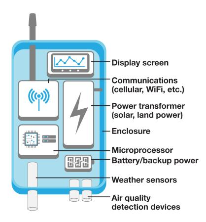
Figure 1-1. Typical Air Sensor Components
