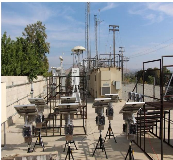
**Figure 4-1. Air Sensors on Tripods (in foreground) with Reference Instruments (in the background) to Evaluate Sensor Performance. Photo Credit: South Coast Air Quality Monitoring District (AQMD)**
