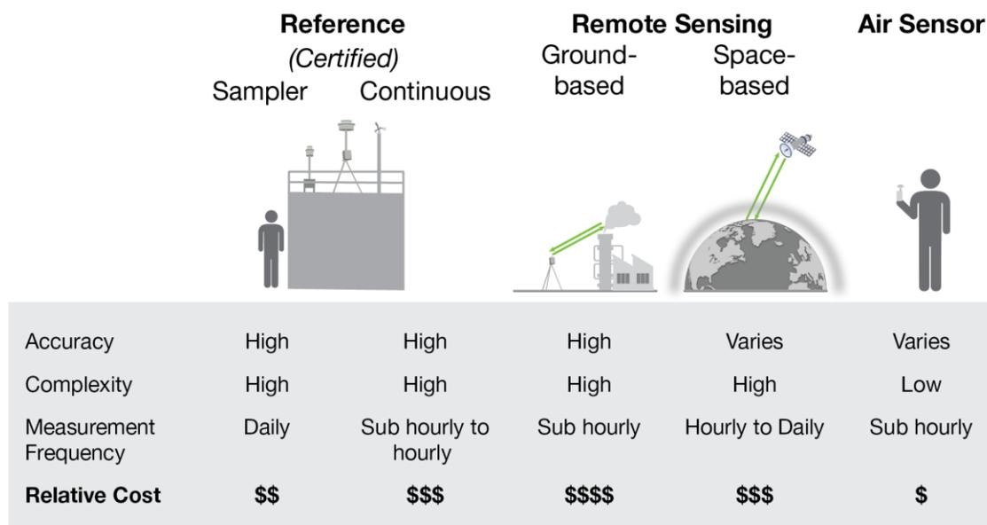
**Figure 2-8. Common Types of Air Monitoring Instruments and Their Characteristics**
