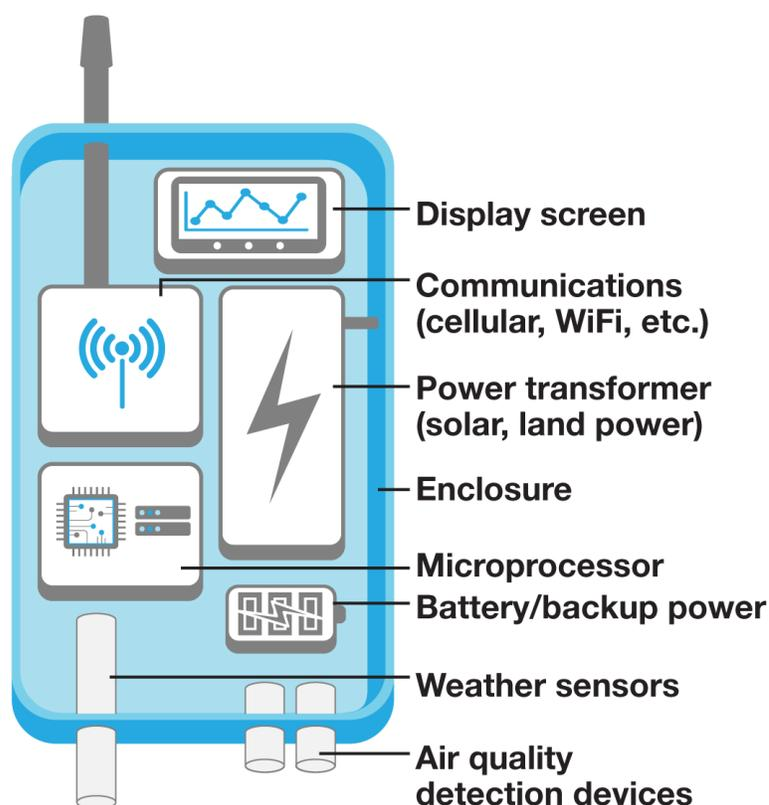
**Figure 1-1. Typical Air Sensor Components**
