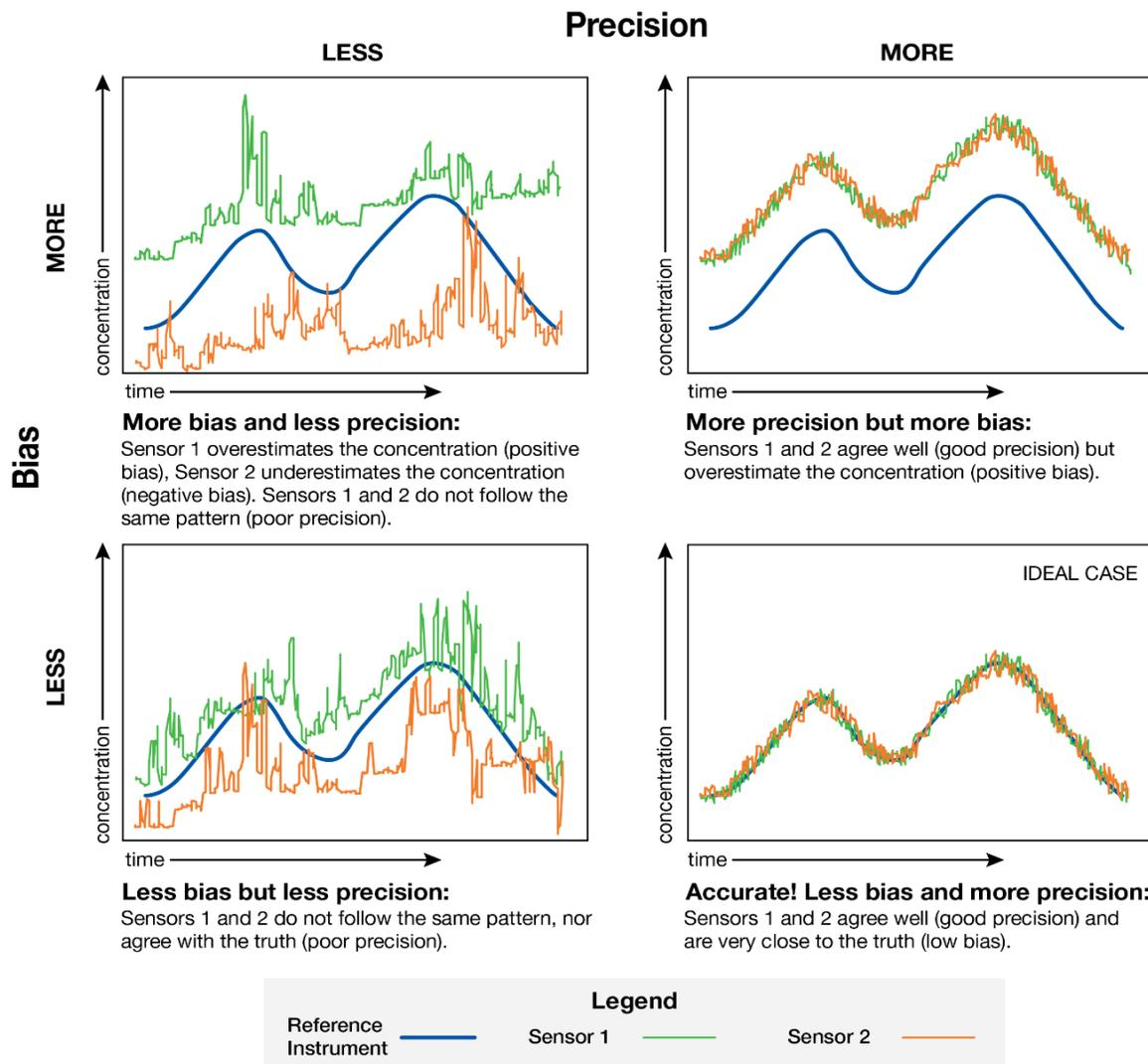
**Figure 3-4. Illustration of Air Sensor Bias, Accuracy, and Precision**
